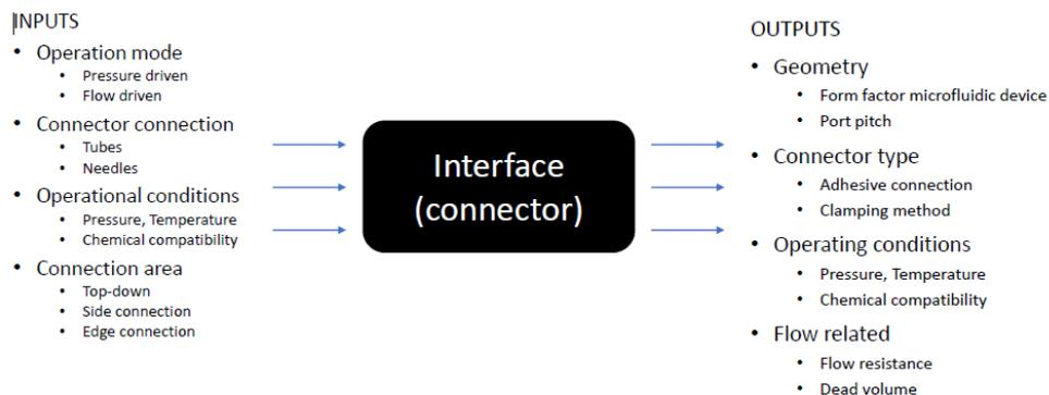
Figure 2: Overview of input and output characteristics for a microfluidic interconnector
