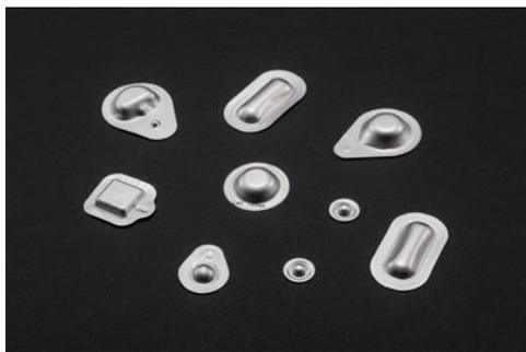
from multiple layers of metal and polymer films with tuned capabilities on chemical resistivity and moisture barriers. The liquid can be released by applying pressure on top of the blister; the foil on the bottom either breaks due to the overpressure or is pushed against a sharp object, puncturing the foil. Technical challenges in implementing blisters include blister design to fit cartridge and reagent volume specification, airfree blister filling, reproducible blister rupture, controlled
